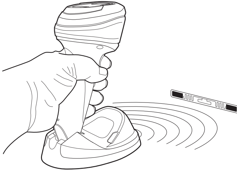
Figure 5 RFID in Hand-Held Mode
